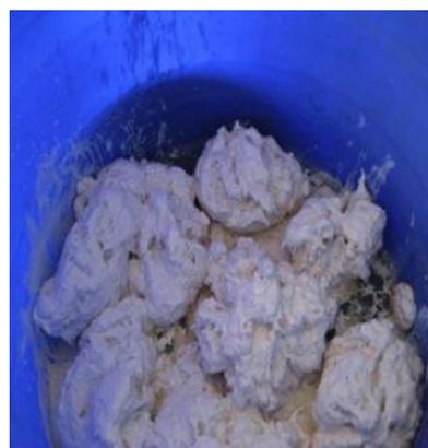
Resulting sludge containing rubber solids collected from processing equipment (Photo: MTEC)
